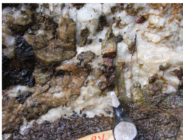
Fig. 13: Photo taken in lower Pettersgruva. The black crystals are clinopyroxene, the white are marble and the grey/beige are scapolite crystals.
