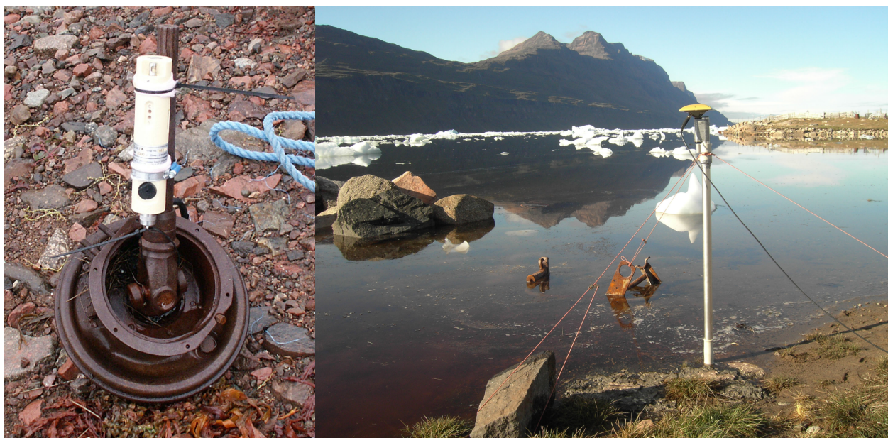
Figure 4. A tide gauge attached to a metal piece (“anchor”) was used to measure the tidal range outside Tasiusaq (left). (Photo: Charlotte Sparrenbom) The portable unit in the GPS-equipment was used to measure the height of e.g. the sea-level and basin thresholds in the study area (right). (Photo: author)
