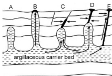
Fig. 5. Basic mud volcano formation. A - clay diapir. B - sea-floor-piercing clay diapir - a mud volcano. C - sea-floor seepage. D, E - mud volcanoes formed due to rise of fluidized sediments along faults. Adopted from Milkov (2000).
