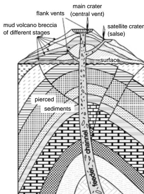
Fig. 3. Basic structure and main elements of a conical mud volcano. Adopted from Dimitrov (2002).
