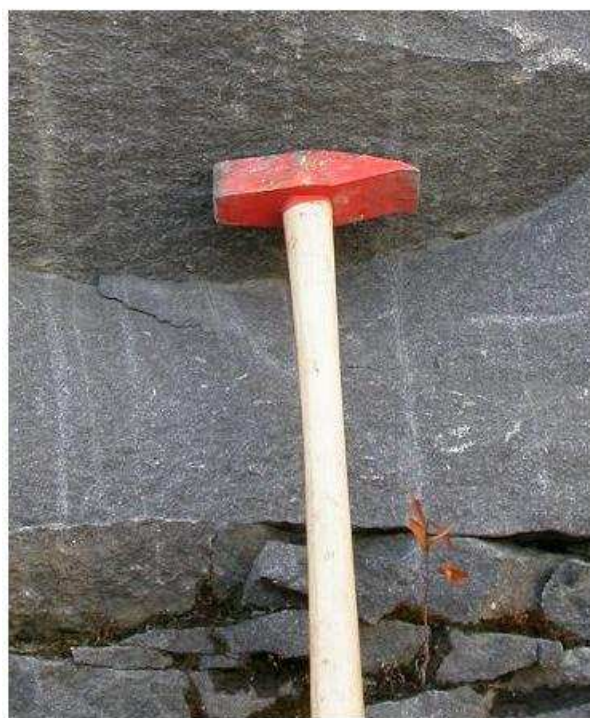
Figure 4. The photo is from the Åkerberg open cut mine. Note the vertical quartz veins, which are characteristic for the gold mineralization in the ore zone.
