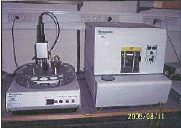
Fig. 10. SediGraph 5120 Particle Size Analysis System, Micromeritics used for the determination of the grain size distribution between 0.063 and 0.001 mm.
