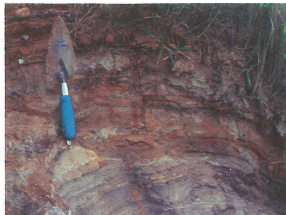
Figure 13b. The northernmost part of the sedimentary unit shown in Figure 12a. The exact location of the photo is indicated in Figure 6. Here the sediments are approximately 20 cm thick, extending from the nail at the base of the trowel to next highest nail. The sediments consist of compact gray clay with interbedded layers of orange sand. No boulders are present in the unit in this area (Photo: Jessica Oster).
