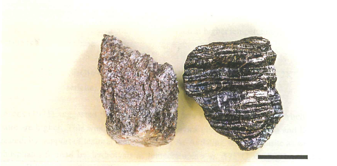
Fig. 22. Samples taken from the tailings of the Västanå mine. Sample to the left is mainly constituted by muscovite/pyrophyllite while hematite is subordinate. Sample to the right is dominated by crenulated specular hematite. (Scale is 3 cm)
