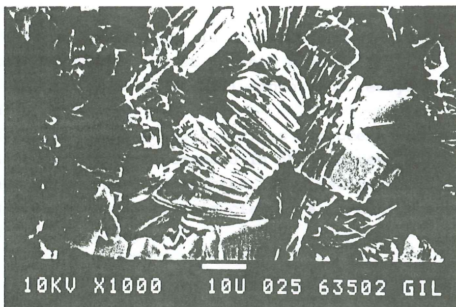
Fig. 11. SEM picture of authigenic kaolinite with characteristic pseudo-hexagonal crystals, forming curved vermicular stacks.
