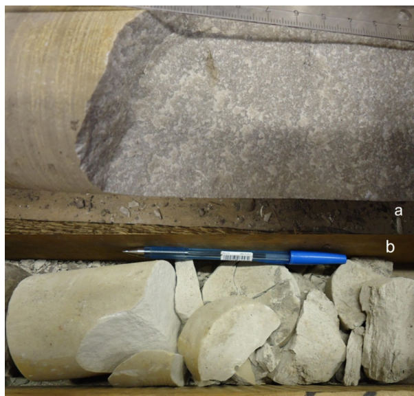
Fig. 14 a & b. Photographs of the sandstone facies 4 in the Höllviken-2 core showing variable degree of consolidation, from the Sinemurian (1380m) and the Uppermost Rhaetian (1435m) respectively.
