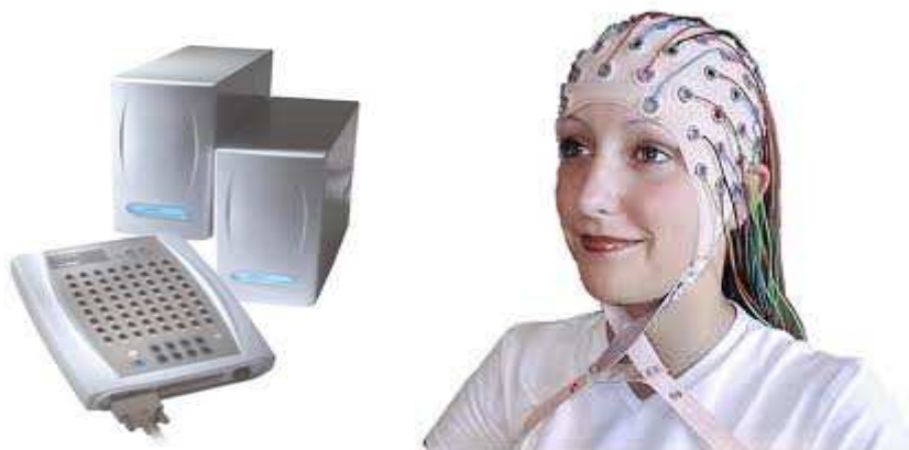
Figure 3 Synamps 2 amplifier and NeuroScan EasyCap
