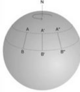
Figure 4.5: As the Earth rotates, the projected baseline will change. Each such projected baseline represents a point in the Fourier plane. By having many pairs of telescopes, it is possible to cover a large part of the Fourier plane simply by making use of the Earth's rotation.
