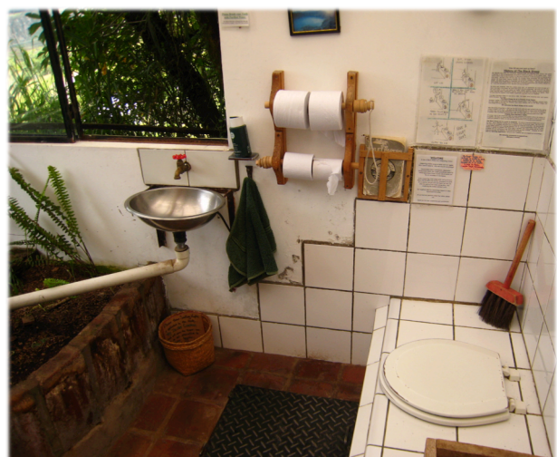
Figure 9. Inside one of the restrooms with composting toilets at Black Sheep Inn. Notice the sink that receives its water from a barrel with harvested rainwater on the roof of the building. Biodegradable soap is provided next to the sink and the grey water is directly transported to the indoor flowerbed; all made clearly visible to the visitor. Information on how the composting toilet works and its many advantages are posted on the wall next to the seat.
