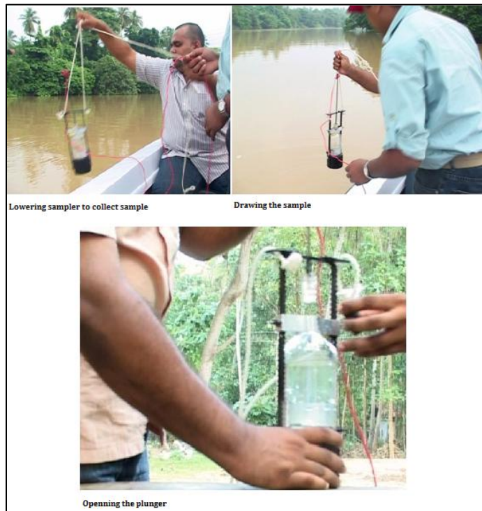
FIGURE 2: COLLECTING SAMPLE FOR SALINITY MEASUREMENTS
