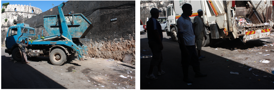
Figure 7. A skip truck and a compressor truck in Stone Town the 20th of February 2012.
