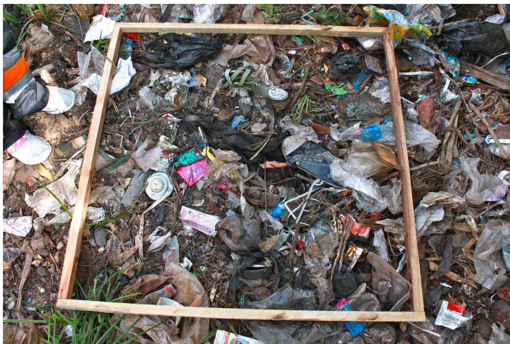
Figure 12. The frame used for the waste composition analysis.
