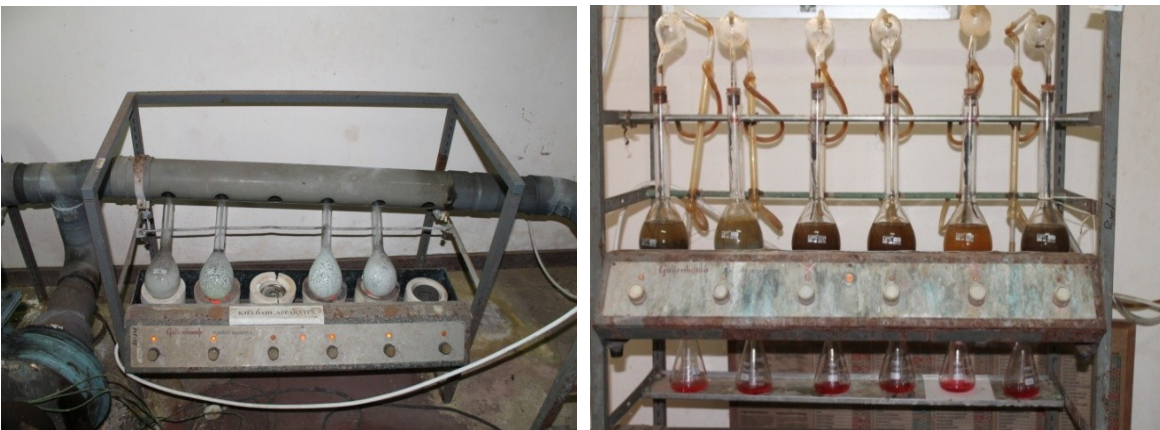
Figure 9. The machines used in the macro-Kjeldahl method. Digesting unit to the left and distilling unit to the right. (Photo: Carolina Emanuelsson and Elna Rasmusson)
