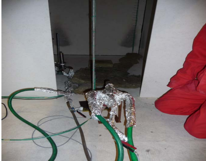
Figure 6- Installation of experimental equipment, Radiometer pointing towards the flame
