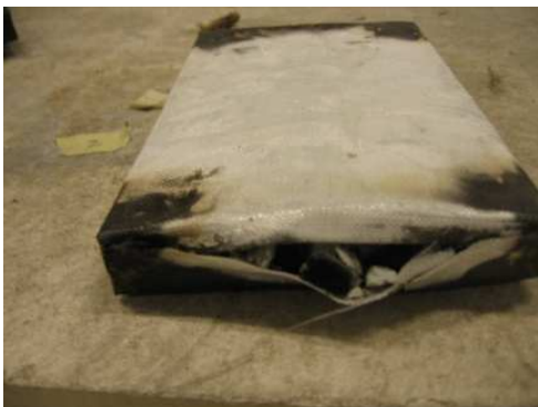
Figure 6.11: Photos of the samples after the tests. a) Test sample 2. Exposed to 40 kW/m 2 . Exposed side; b) Test sample 6. Exposed to 48 kW/m 2 . Unexposed side.
