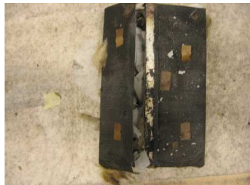
Figure 6.11: Photos of the samples after the tests. a) Test sample 2. Exposed to 40 kW/m 2 . Exposed side; b) Test sample 6. Exposed to 48 kW/m 2 . Unexposed side.
