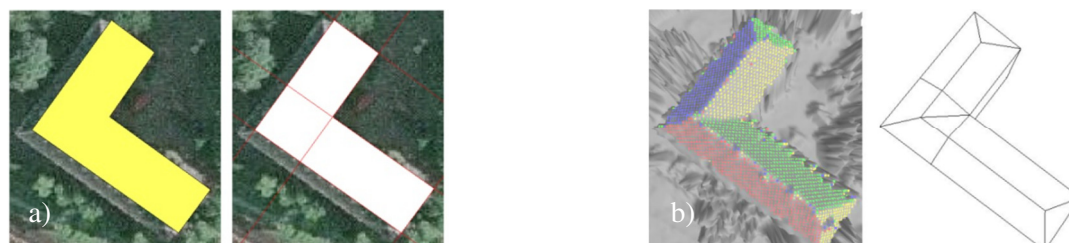
Figure 13. a) Building footprint and its decomposition into cells. b) LiDAR points inside the cell colored according to their local regression plane and the best fitting roof shapes.
