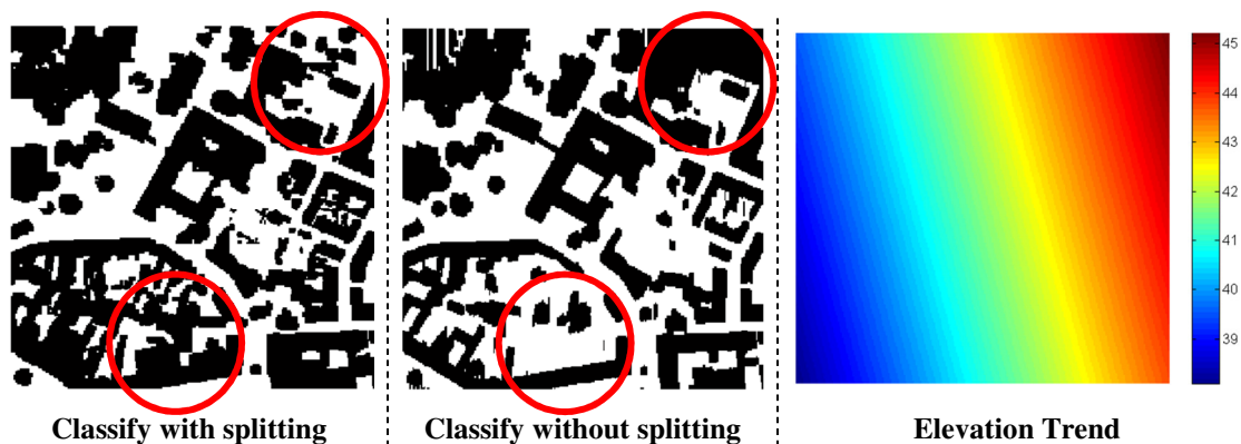
Figure 40. The comparison of classifications of ground and non-ground areas with and without being split beforehand, and the estimated elevation trend.
