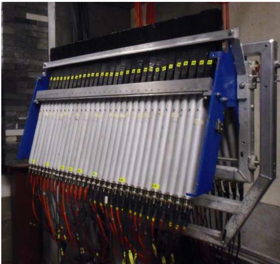
Figure 9. Photo of the hodoscope. In the figure, the black sticks are the wrapped scintillators and light guides and the metallic tubes contain the PMTs [8].
