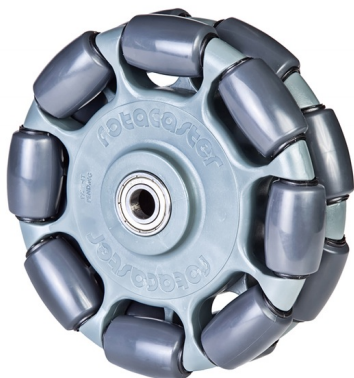
Figure 2: Picture of an omni-wheel which can roll both in "normal wheel direction" and perpendicular to it due to the extra rollers along the wheel.
