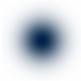
Figure A.1: The beam intensity of a cross section of a fundamental Gaussian beam for a chosen w(0) and w(z) .
