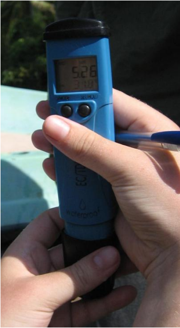
Figure 18: The salinity meter used in the field measurements. Water samples were taken at different depths and the salinity was measured for each sample.
