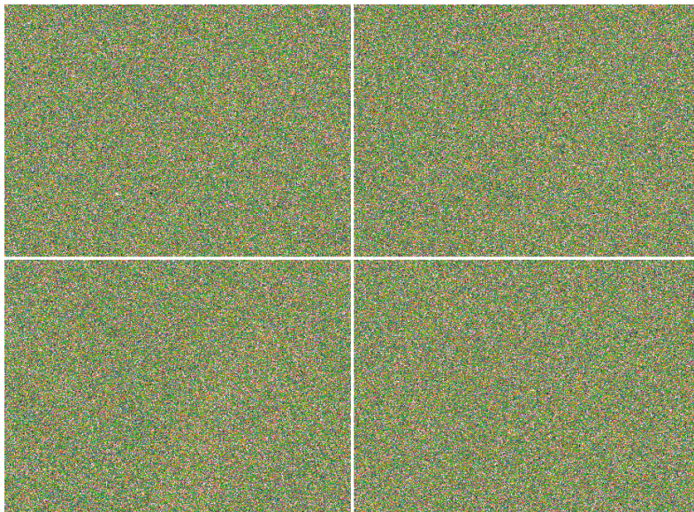
Figure C.6: Percent difference images from flatfield session JD 2455831. Left to right: IRCUT \Delta t 13.6min, VE1 \Delta t 6.5min, VE2 \Delta t 5.4min, V \Delta t 0.7. The images have been histogram equalized and coloured to emphasize that there is no discernible structure.
