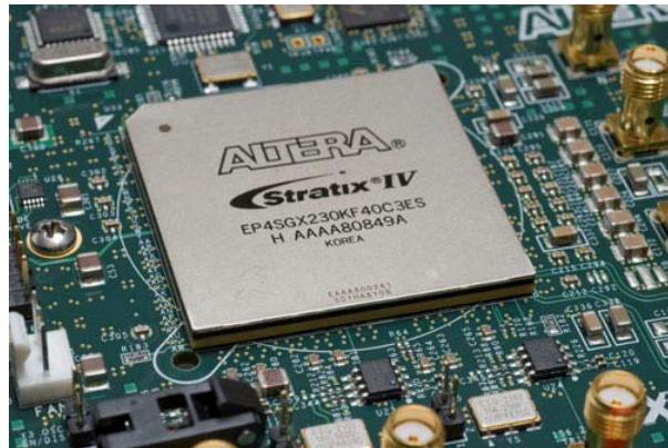
Fig. 2.4 – Example of an Altera Stratix IV GX FPGA [14]
