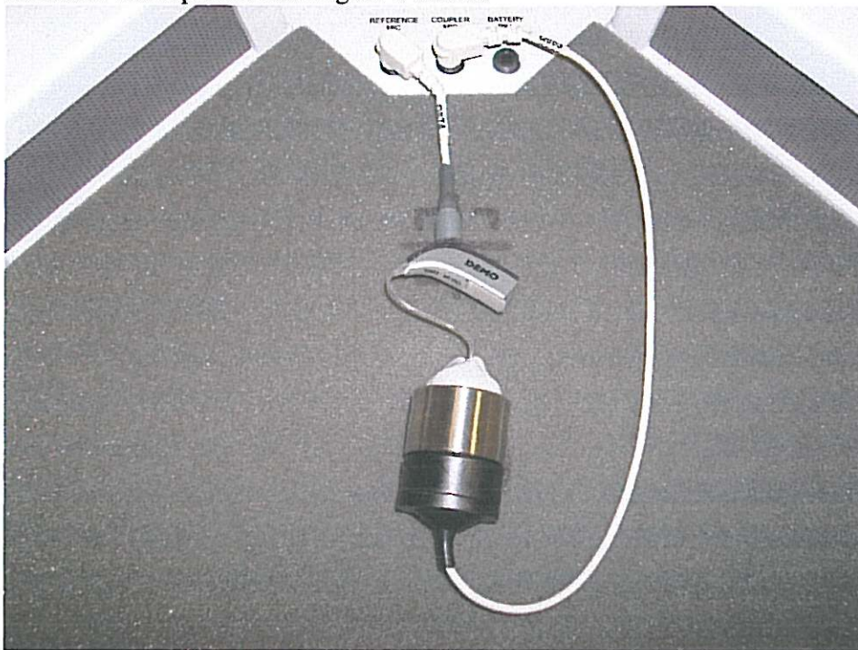
Figure 2. The test set-up for electro acoustic measurements on one hearing aid.
