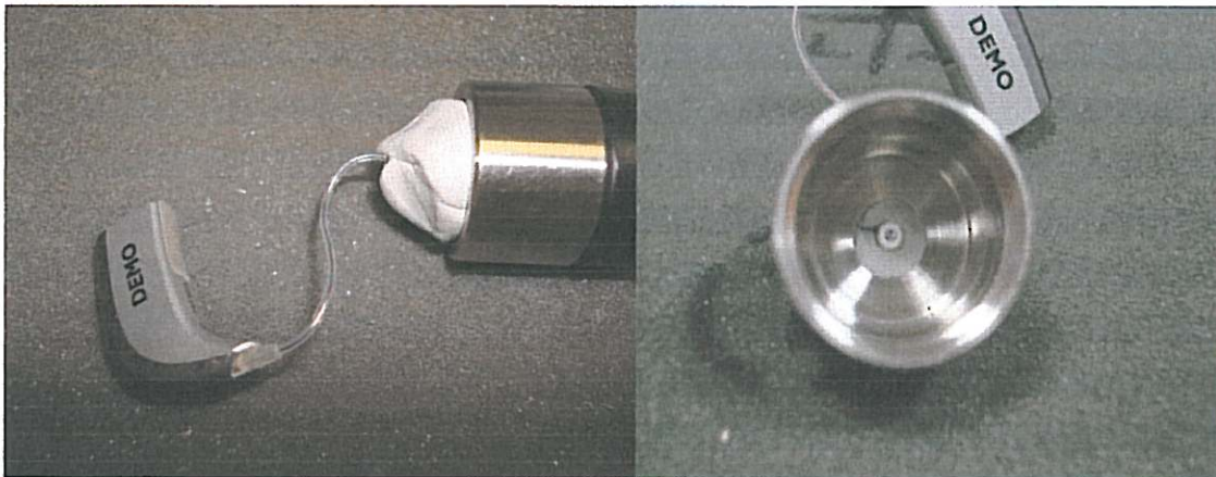
Figure 3 and 4. Shows how the hearing aid's receiver was connected to the coupler.
