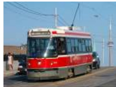
Figure 15 – Toronto streetcar have cutouts that resemble wheel wells on buses.
