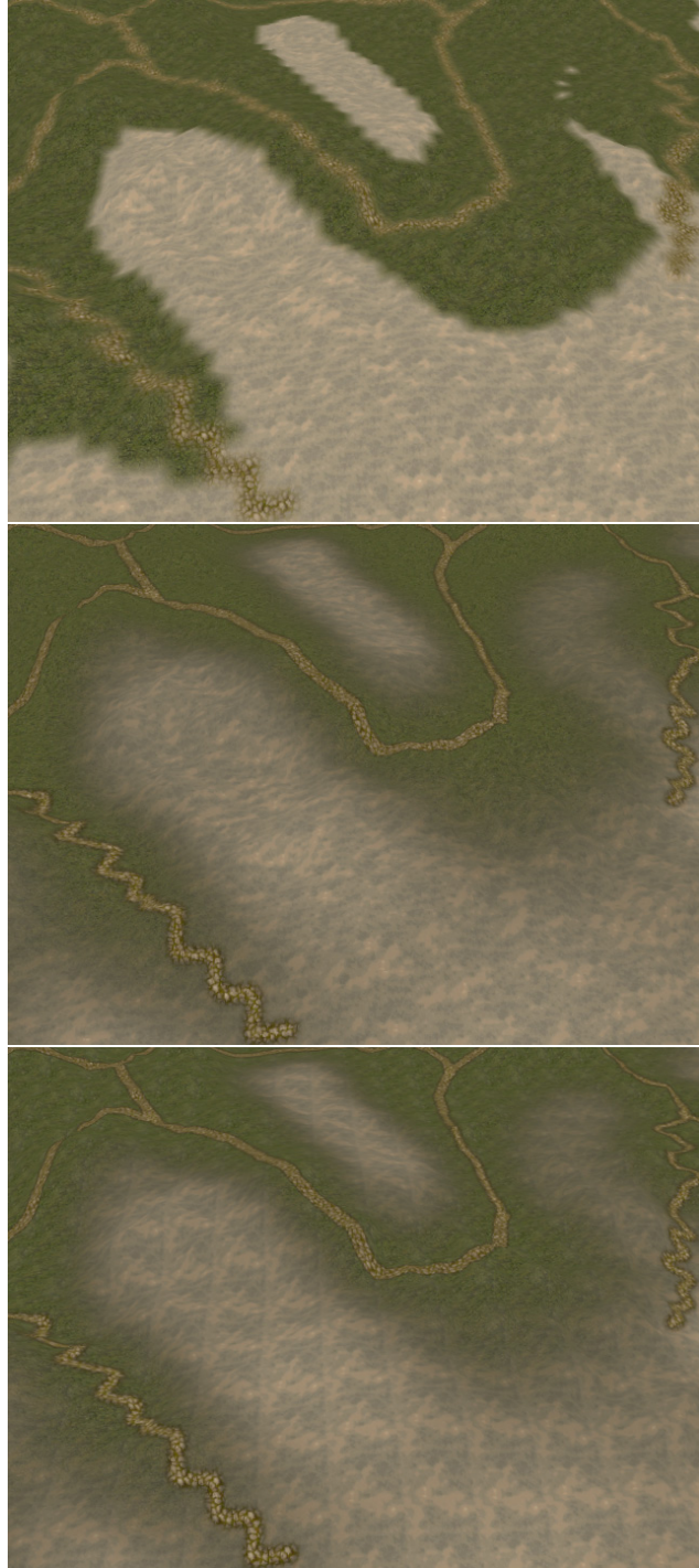
Figure 11: A visual comparison of the different multi-texturing techniques. The top-most image uses the texture-array based shader, the middle image uses synthesized texture splatting and the bottom images uses regular splatting.
