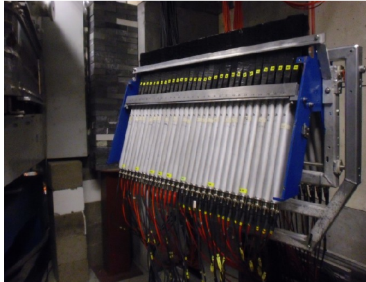
Figure 1.6: Focal-plane hodoscope used at MAX-lab. There are two sets of PMTs, each set belonging to one of the two scintillator planes.
