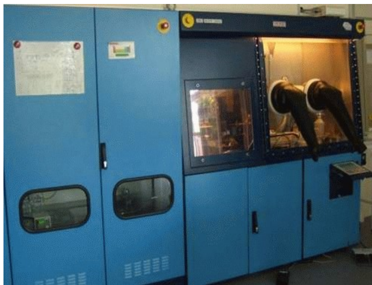
Figure 2.1- Aixtron AIX 200/4, used for MOVPE growth of nanowires at Lund Nanolab (picture courtesy of www.nano.lth.se )
