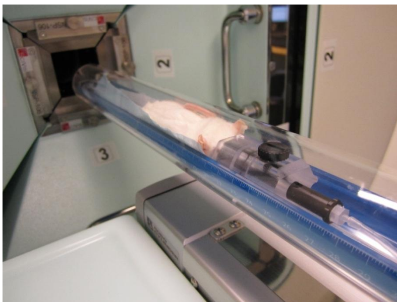
Figure 3.10 An NMRI mouse prior to imaging. The mouse is provided with a sufficient flow of isoflourane to keep it anaesthetized and warm air to keep the body temperature stabilized.
