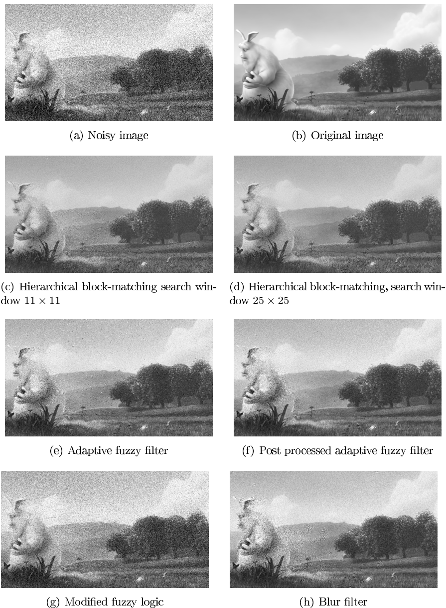
Figure 8.3: Frame 2323 from the Big Buck Bunny sequence filtered using a few of our methods. The added noise has standard deviation \sigma = 40 .
