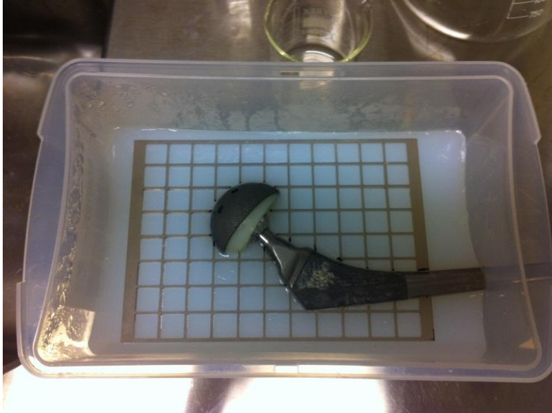
Figure 3.1.2 The Omnifit prosthesis with half the container filled with agarose gel and the rectilinear grid put in place.
