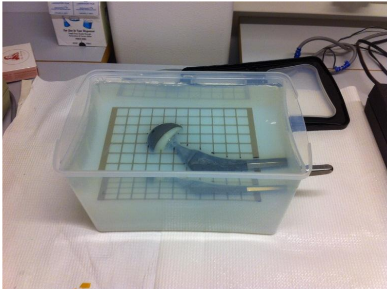
Figure 3.1.2 The Omnifit prosthesis phantom complete with the top layer of agarose gel still waiting to harden.
