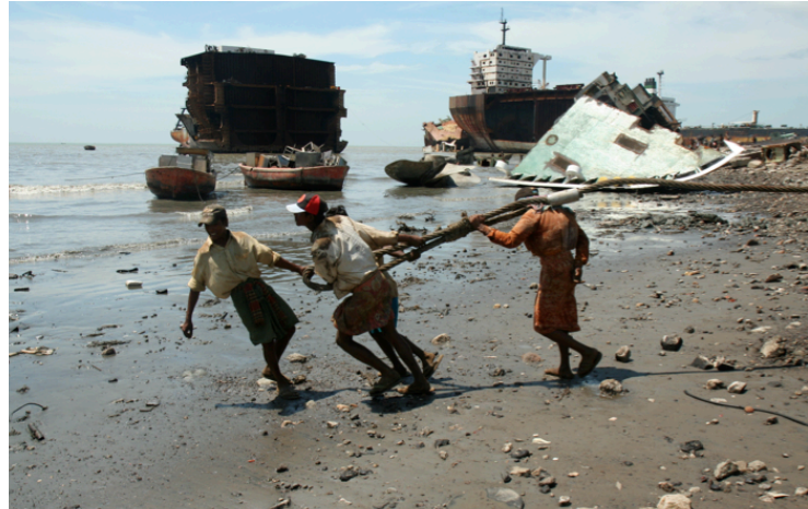
Figure 2-8 Ships broken by beaching method; A large steel block is being dragging by human forces in Chittagong, Bangladesh
