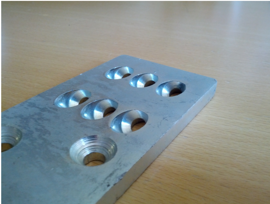
Figure 5.3.2: Example to inclined pre-drilled holes in the steel plate to host the head of the screws
