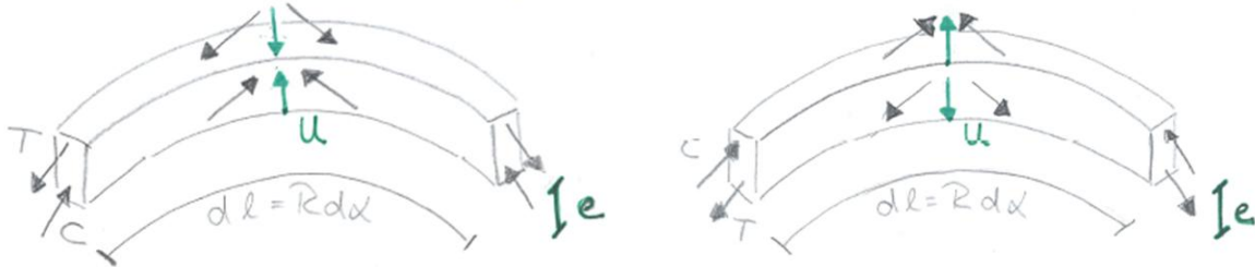
Figure 4.24 Global view of the radial deviation forces u along an element with the length dl
