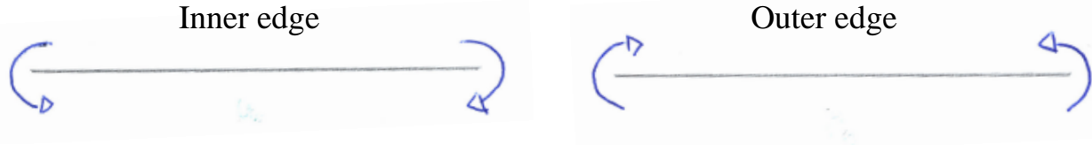
Figure 4.22 Simple demonstration of the deck's bending moment depending on inside (left) or outside (right) suspension
