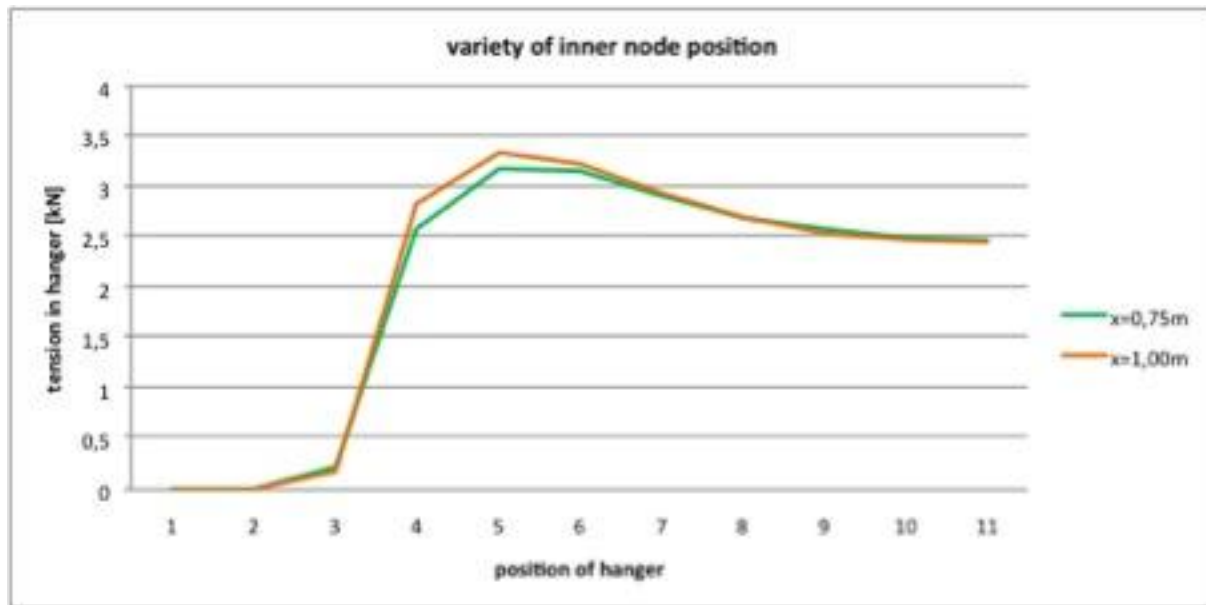
Figure 5.27 Tension in the hangers: inner node case x=0,75\text{m} compared to inner node case x=1,00\text{m} ; \varphi = 45^\circ
