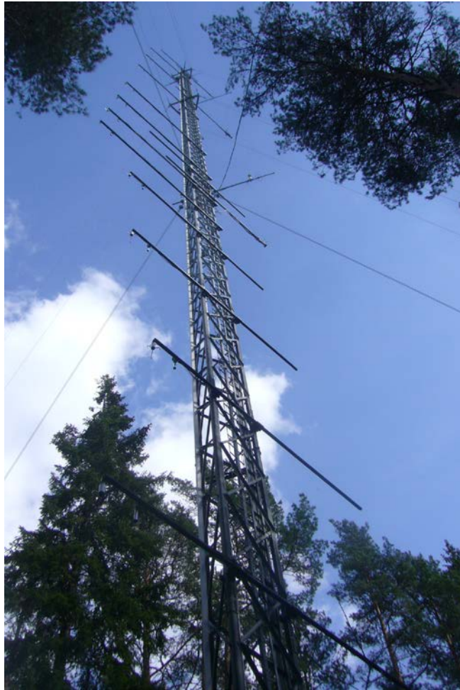
An eddy covariance tower in Norunda (Sweden). Credit photo: Sarah Loudin
