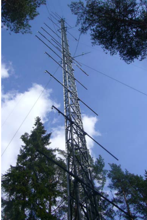
Figure1: photo of an eddy covariance tower in Norunda, Sweden (Sarah Loudin).
