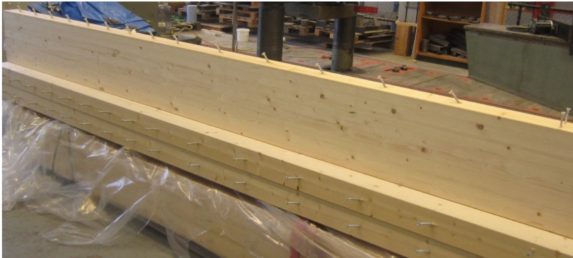
Figure 4.8: Timber beams with inserted the screws at an angle of 45 degree.
