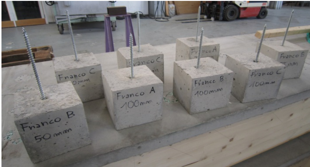
Figure 7.42: Samples for the withdrawal test with three different depth of anchor.
