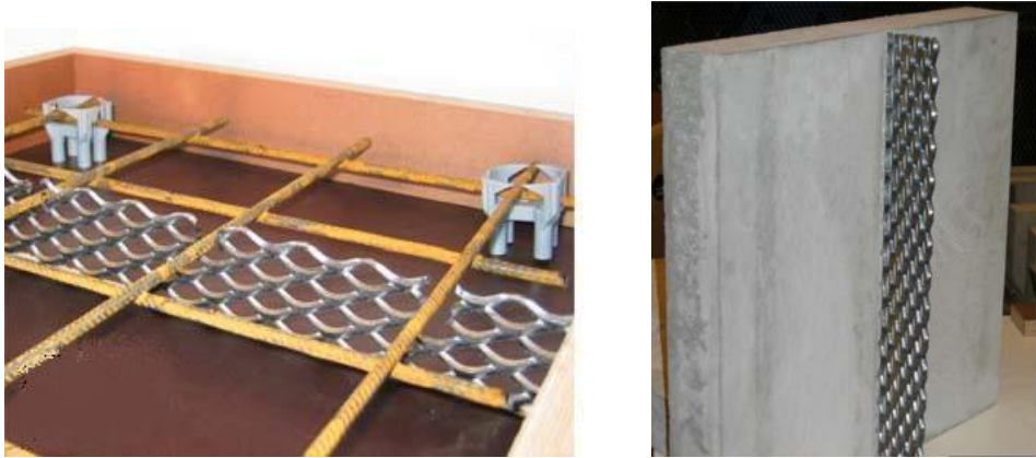
Figure 2.4: Epoxy-glued connections in the moulding forms continuous steel mesh (SM) on the left. Prefabricated concrete slab with inserted shear connector on the right, see [1].
