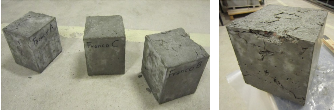
Figure 7.41: Concrete cubes after the compressive test.
