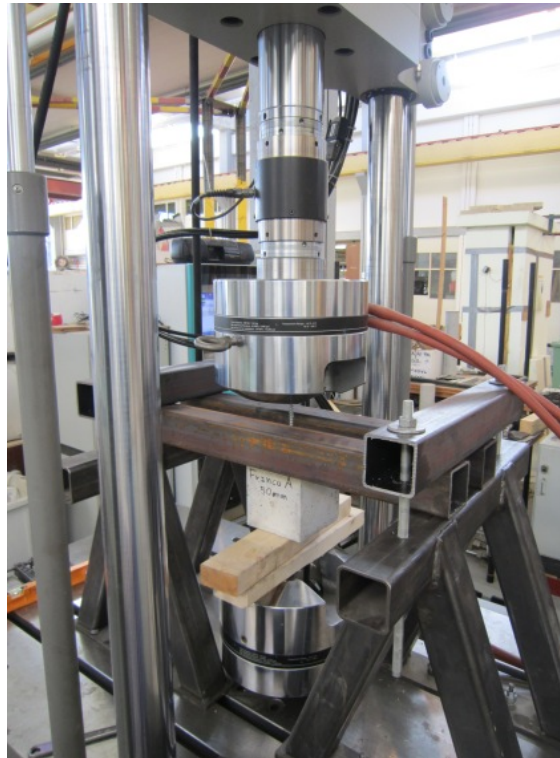
Figure 7.43: Machine and steel frame used to perform of the withdrawal test.
