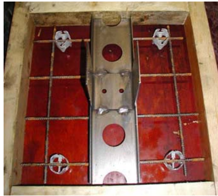
Figure 2.10: SP+N* shear connector type in moulding form, see [1].
