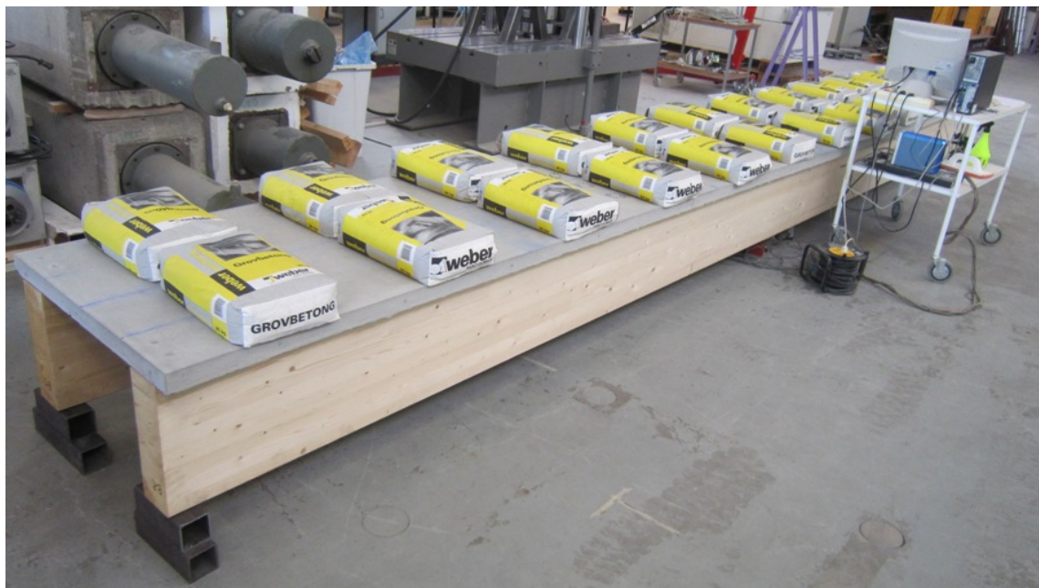
Figure 7.38: Full-scale specimen B loaded by 100 kg/m 2 for long-term test.
