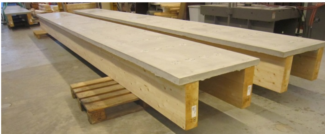
Figure 4.17: Composite beams stored in the laboratory of Lund.
