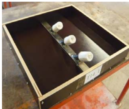
Figure 2.16: Steel tubes in the formwork before concrete casting.
