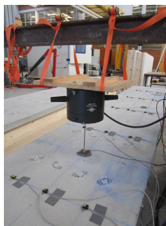
Figure 7.2: The shaker and the accelerometers surrounding it.
