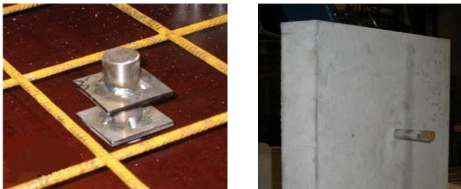
Figure 2.6: Epoxy-glued steel dowel with flanges (GDF), the moulding form on the left. Prefabricated slab with inserted shear connector on the right, see [1].
