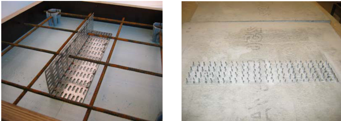
Figure 2.3: Toothed metal plate connector (Type SNP), in the moulding form on the left and the prefabricated slab with inserted the metal plate on the right.
