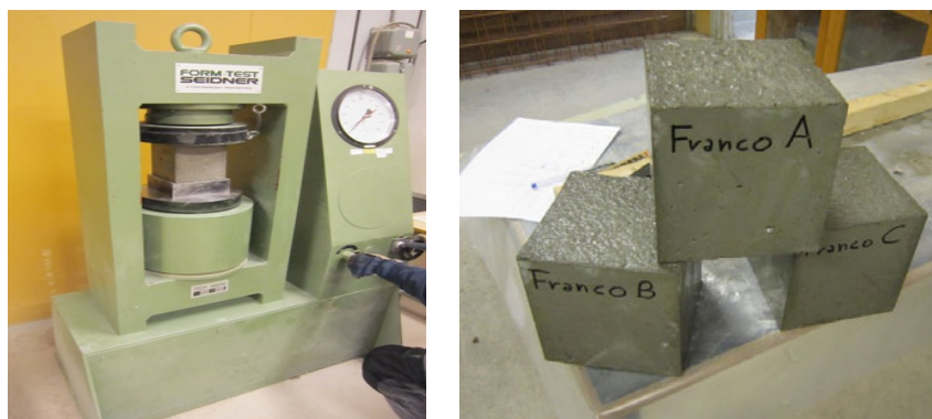
Figure 7.40: Uniaxial compression failure test and cubic specimens before the compressive test.
