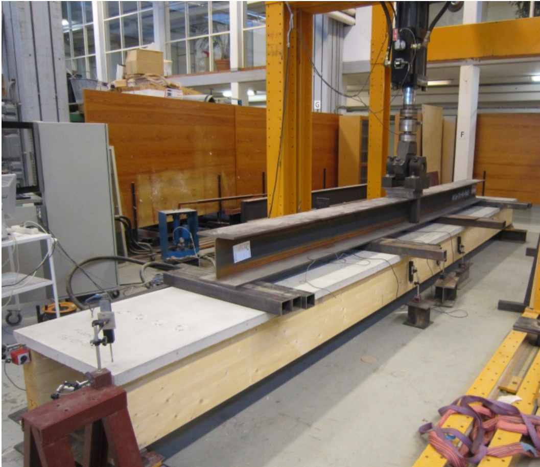
Figure 7.9: Equipment used to perform the bending tests.
