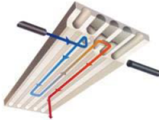
Figur 9 TermoDecks system (Adl-Zarrabi et al., 2011).
