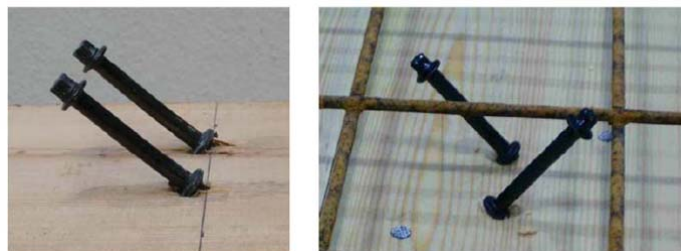
Figure 13: SFS VB screws in an inclined arrangement in the longitudinal direction (Jorge 2005)
