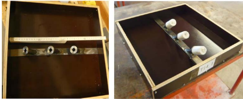
Figure 72: beam to slab connection system type T12 used for the researches described in Paper [1]
