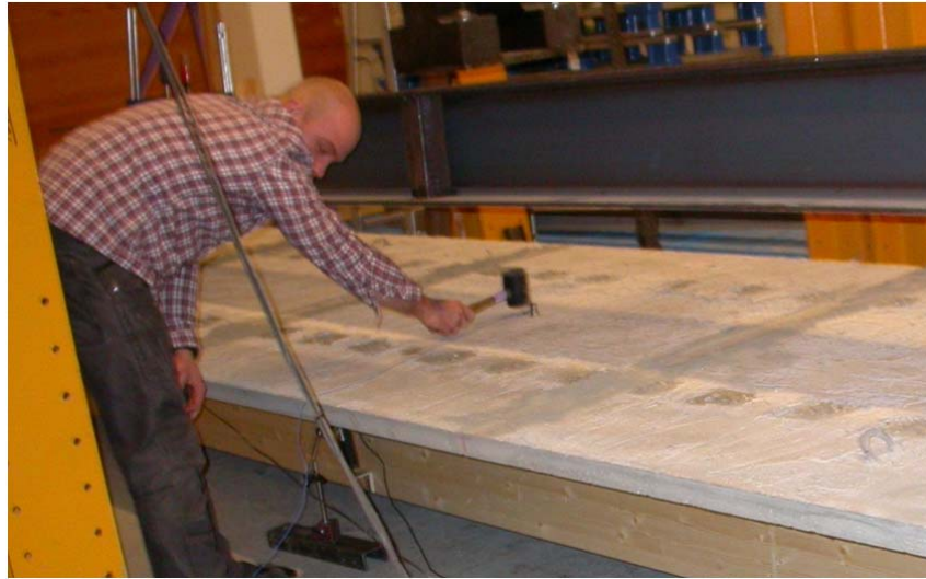
Fig. 103: excitation of the system by using an hammer in order to induce vibrations
