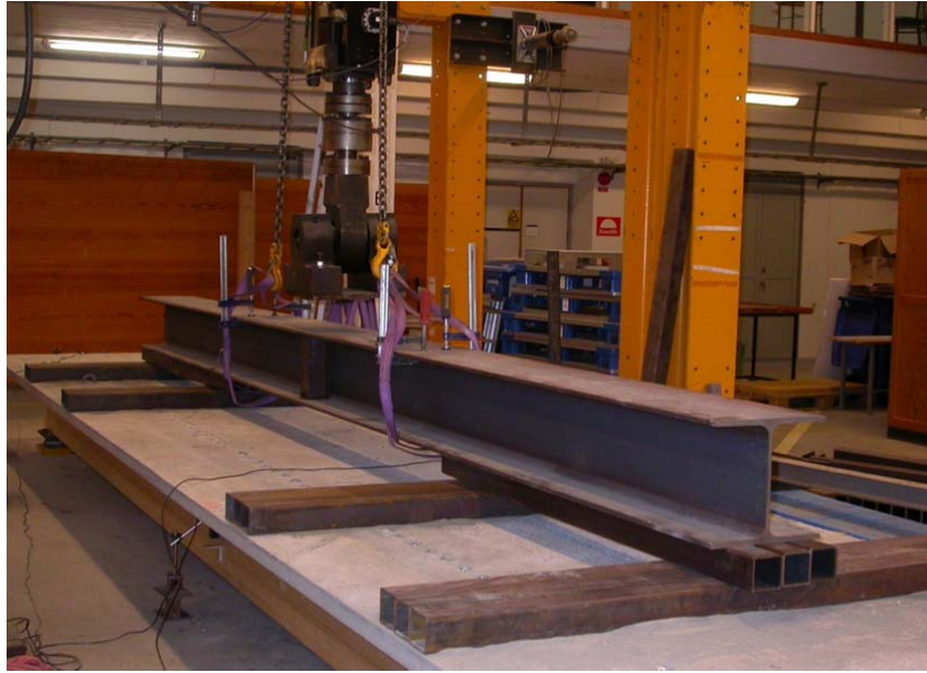
Fig. 101: equipment used to perform the bending tests
