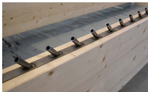
Figure 77: steel plate with welded pipes containing the screws (used in the tests of this Paper)
