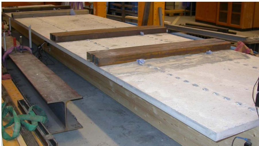
Figure 125: commercial background type specimen before the bending tests
