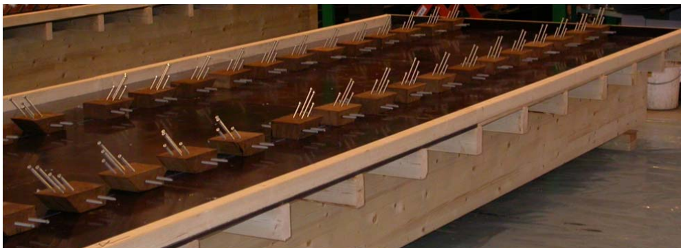
Figure 86: furfurylated wood pieces in the formwork (tests of this Paper)
