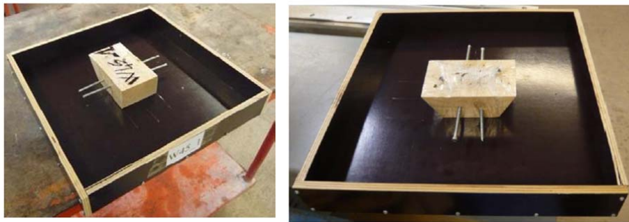
Figure 85: furfurylated wood pieces in the formwork (Paper [1])
