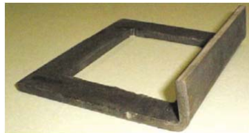
Fig. 50: overall view of bent plate connector
