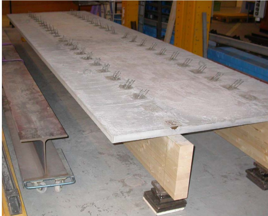
Figure 110: residential background type specimen before the bending tests
