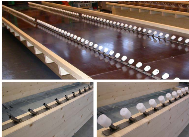
Figure 73: beam to slab connection system type T12 used for the experimental researches described in this Paper
