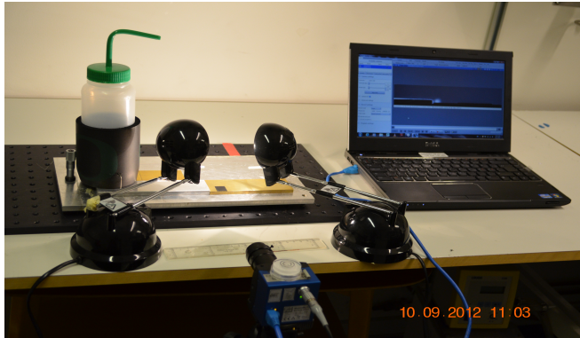
Figure 4.2: A picture of the experimental setup which is used for liquid nitrogen droplets.
