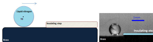
Figure 6.3: A liquid nitrogen droplet in the film boiling regime moves toward an insulating step, which is lower than its radius.
