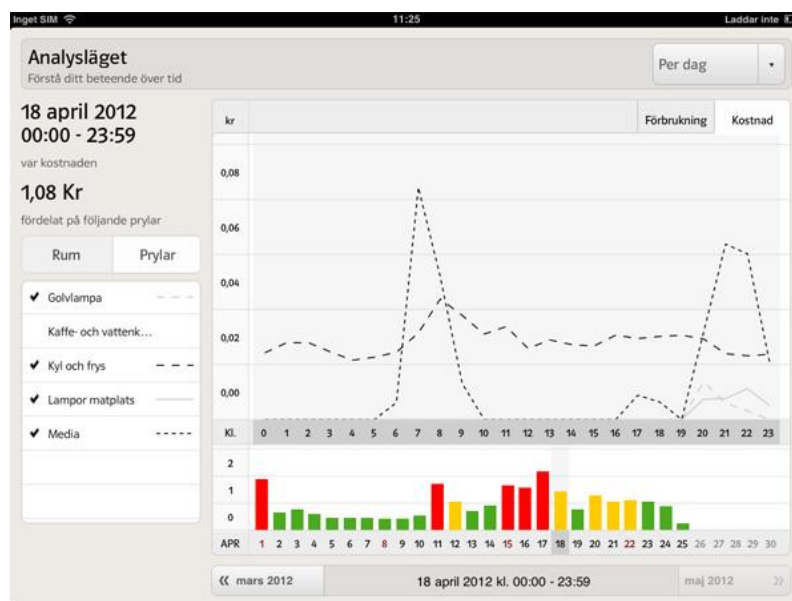
Figure 9. Analysis Mode. Upper chart is showing cost feedback for one day. Lower chart is showing power use for one month.
