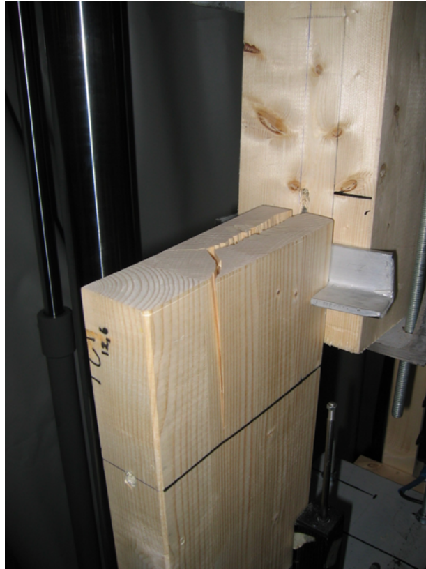
Figure 5.7: Splitting failure in side-member, test 90°,6.
