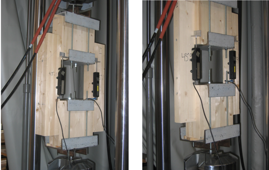
Figure 5.12: Test set up when examining a_{3,t} (left) and a_{4,c} (right) in joints with inclined tension screws.
