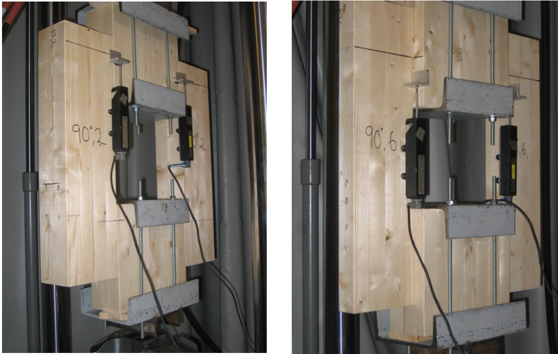
Figure 5.6: Test setup when examining a_{3,t} (left) and a_{4,c} (right) in joints with laterally loaded screws.
