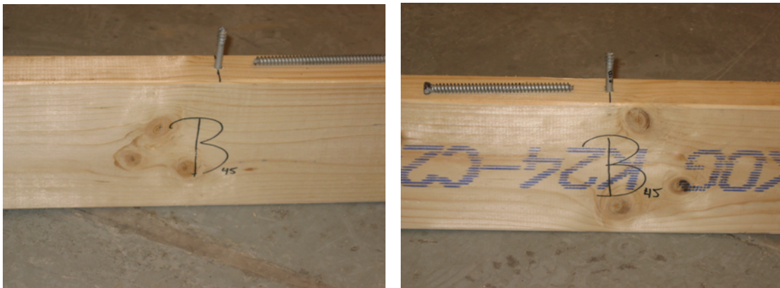
Figure 5.3: Test piece B 45 . Screw failure.
