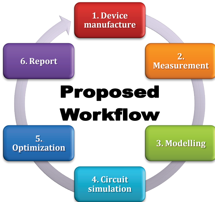
Figure 1 – Proposed workflow, from device manufacture to report generation. All steps excluding 1 and 2 are implemented in the developed software and are highly automated.
