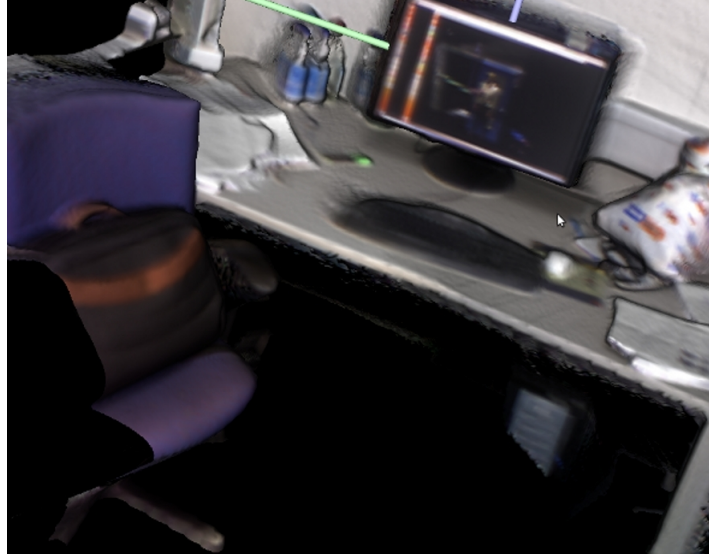
Figure 5.6: Using point-to-plane and a running average of the colours, this 3D reconstruction is obtained. If one looks at the screen one can see another 3D reconstruction of the author.
