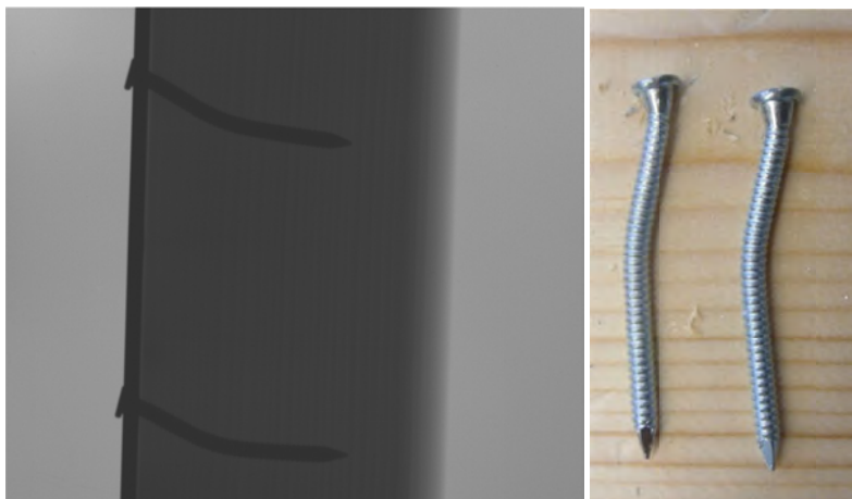
Figure 17: X-ray image at high load, 4d-2.5-n60, two plastic hinges visible.
