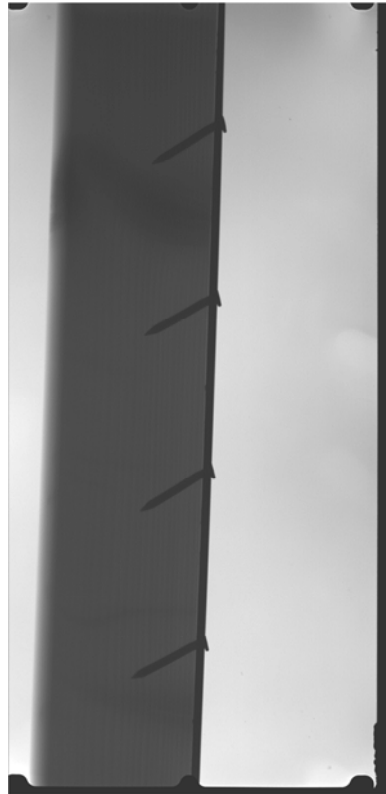
Figure 16: X-ray picture at maximum load on the 4d-2.5.n40 series, one plastic hinge formed at the steel timber interface.
