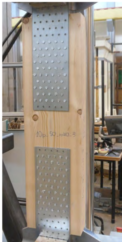
Figure 1: Mechanical steel to timber joint with nail type fasteners.
