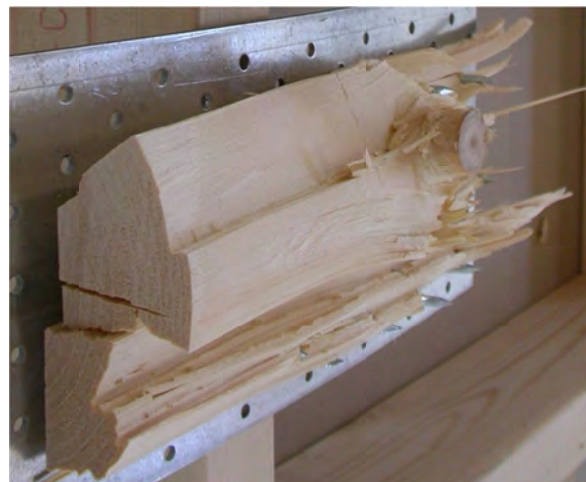
Figure 28: Plug shear failure in one of the specimens, 3py-5-n40 series.
