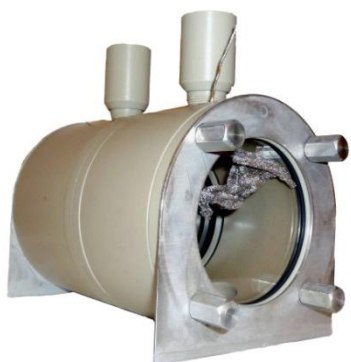
Figure 7 In-house developed chamber for anodization of silicon wafers.
