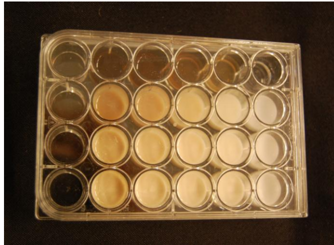
Figure 4. 4: A photo of the type of well plate used, with the different mixtures of water, blood and Intralipid in the different wells.
