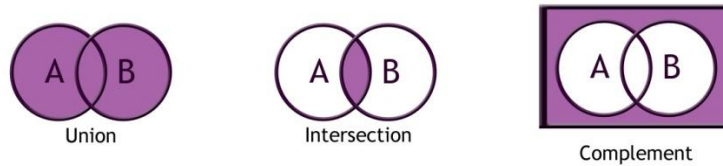
Figure 3.1. The cells could be defined as union, intersection or complement of regions bounded by surfaces.. For this the schematic illustration, circles in two-dimensional space are used as a simple example.
