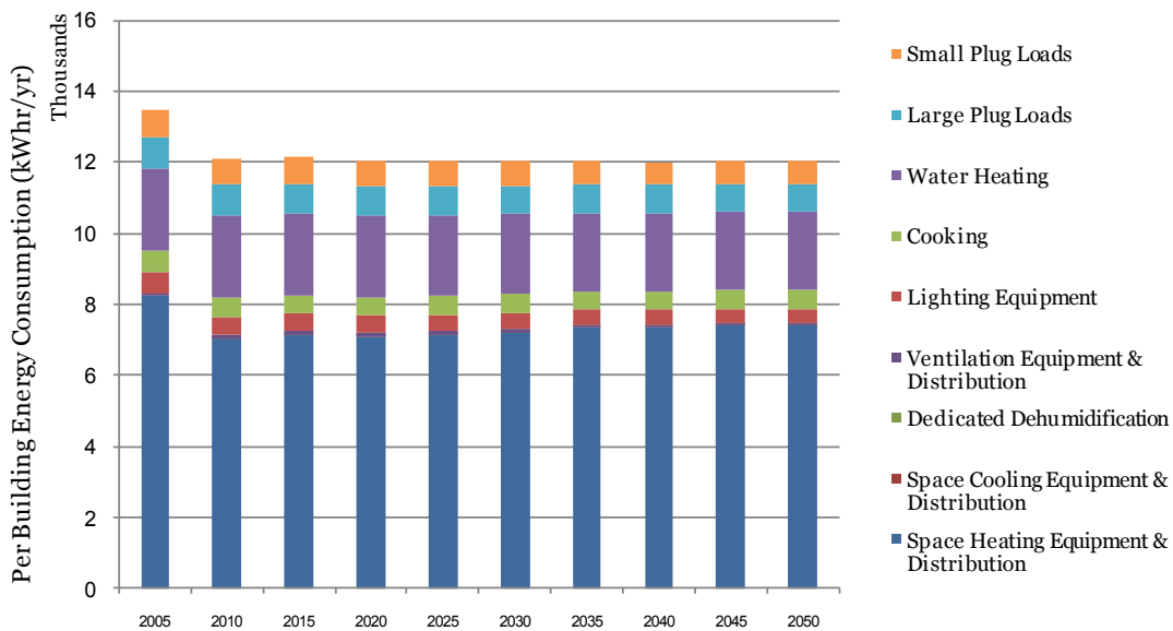
Figure 3- 16: Per building energy consumption according to policy scenario 5 – Incentives combined with current Swedish energy policy.
