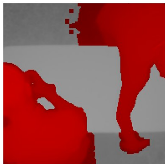
Figure 3.3: Foreground segmentation where a low threshold was used for the entire image. Areas over the counter are accurately segmented whereas the noise around it is unmistakably higher.
