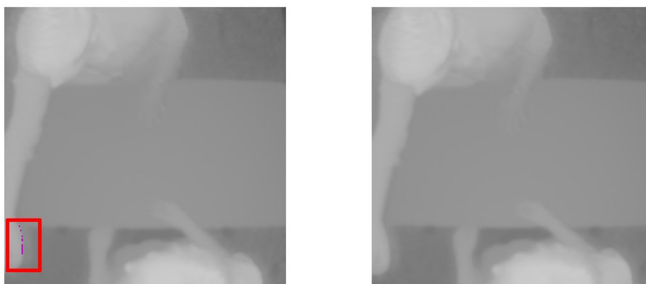
Figure 4.16: Left image shows a false alarm due to noise along the edges of the customer's hand. The right image shows the same scenario where the falsely classified pixels have been removed with a morphological opening.
